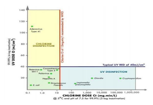
Diagram: Efficacy levels of chlorination and UV in the inactivation of various viruses (EPA).
